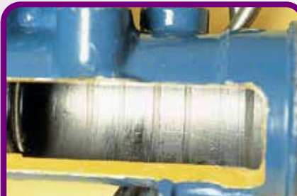
Grooves are worn into the soft metal of the spool valve housing by hardened seals.
