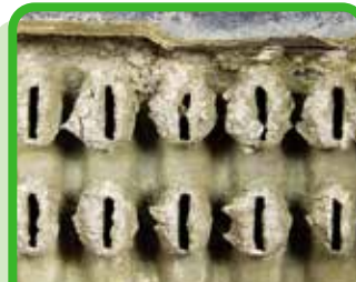
Rust, scale and sludge can plug cooling system fins, preventing proper circulation of coolant.
