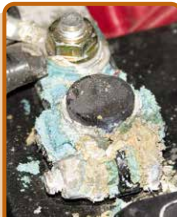
Battery terminal with corrosion buildup.
