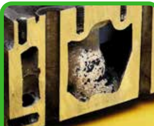
Severe corrosion can occur when additives have been depleted.
