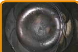
BEFORE: Piston with heavy buildup of carbon deposits.
