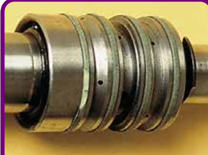
Power steering spool valve with hardened, cracked seals.
