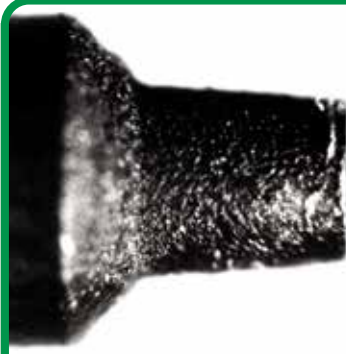
Diesel injector pintle with carbon buildup.
