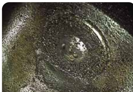
BEFORE: Fuel injector with heavy buildup of carbon deposits
