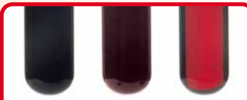
Worn out, oxidized transmission fluid.
