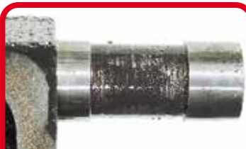
Transmission valve body spool with deposit buildup.
