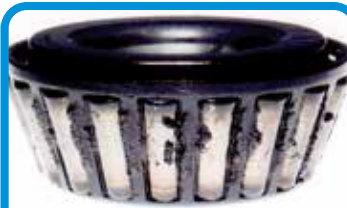
Heavy deposits reduce equipment life.
