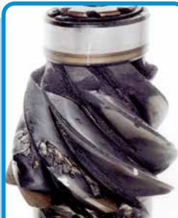
Lubricant breakdown can severely damage critical gear components!
