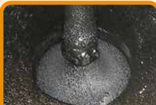
BEFORE: Valve with heavy buildup of carbon deposits.
